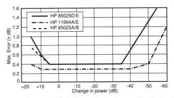
**Note:** For  $\leq$ 20 dB change of power within +10 to -40 dBm the specification for the HP 8757C/E with the HP 11664A/E is  $\pm$  (0.1 dB +0.01 dB/dB).
