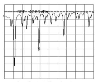
Figure 2. Wavelength calibrator absorption spectrum
