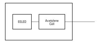
Figure 1. Wavelength calibrator block diagram
