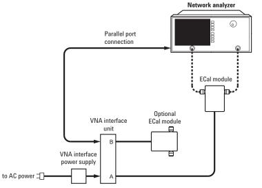
Calibration configuration using the 85097B VNA interface kit
