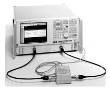
Calibration configuration using the PNA series
