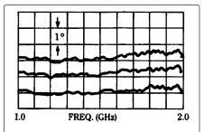
Center trace is phase response of 8491A –6 dB attenuator from 1.0 to 2.0 GHz taken with Agilent 8410 network analyzer. Top and bottom traces are  $\pm 1^{\circ}$  calibration. Linear phase component has been compensated for with a line stretcher. Response, therefore, shows nonlinear phase deviation of  $<\pm 1/2^{\circ}$  over 1 to 2 GHz band.
