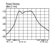
Characteristic output spectrum in the range 1500 to 1600 nm
