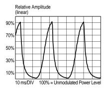
Characteristic output waveform when modulated with 270 Hz square-wave
