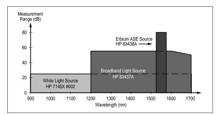
Measurement range of incoherent sources in conjunction with an HP 7145X Optical Spectrum Analyzer at 1 nm resolution bandwidth (RBW). The measurement ranges shown increase and decrease by 10 dB for 10 nm and 0.1 nm RBW.
