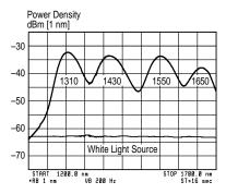
Characteristic spectrum when four EELEDs are installed (HP 83437A with options 003, 004 and 006)
