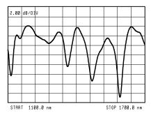
PMD measurement of a 4 km low-PMD fiber on a shipping spool
