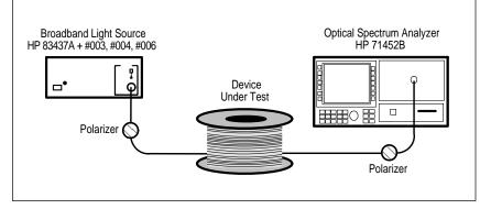
Test setup of a PMD measurement using the wavelength-scanning method.
