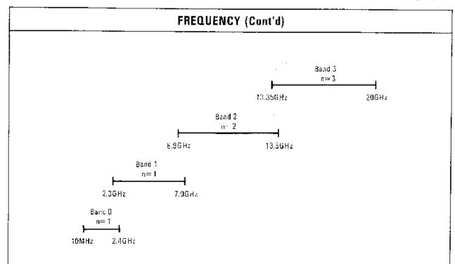
Figure 1. Typical Frequency Ranges and Bandswitch Points in Swept Modes
