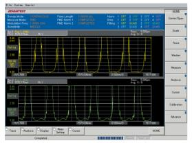
PMD characteristics of interleavers (2-port measurement
