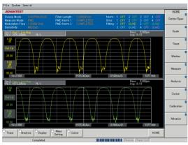
IL characteristics of interleavers (2-port measurement)
