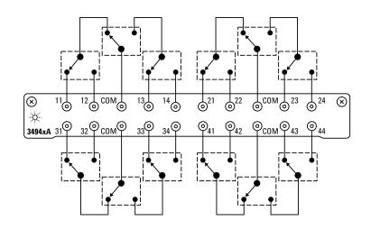
The 34941A and 34942A are configured as four independent 1x4 RF multiplexers on a single module. Multiple banks can be connected together to create a larger multiplexer -up to 97 RF multiplexer channels in a single 34980A mainframe. To prevent ground loops, individual multiplexers are isolated from each other and from the mainframe's chassis. However, the multiplexer channels can be chassis grounded with a simple change. Both 50-ohm and 75-ohm versions are available.
