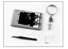
Terminal Connector: 7 mm DUT Connection: 2-Terminal Electrical Length: 11 mm Dimensions (approx.): 150(W) x 70(H) x 90(D) [mm] Weight (approx.): 400 g
