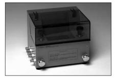
**DUT Connection:** 2-Terminal Bias Voltage Output connector: BNC(f) **Dimensions** (approx.):  $216(W) \ge 173(H) \ge 235(D) \text{ [mm]}$ Weight (approx.): 2500 g **Basic Measurement Accuracy:** 2%(< 1 kHz), 1% (≥ 1 kHz) For detailed information, refer to the operation manual of 42841A.
