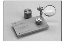
Terminal Connector: 7 mm DUT Connection: 2-Terminal Electrical Length: 26.2 mm Dimensions (approx.): 140(W) x 48(H) x 78(D) [mm] Weight (approx.): 250 g Additional Error:
