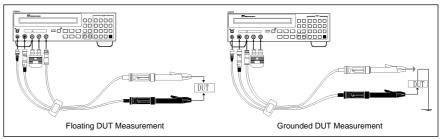
Floating and grounded DUT measurement
