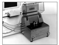
DUT Connection: 2-Terminal Bias Voltage Output connector: BNC(f) Dimensions (approx.): 213(W) x 173(H) x 235(D) [mm] Weight (approx.): 3100 g Basic Measurement Accuracy:  $\sqrt{f}$  [%] + 4285A's accuracy [%] f: [MHz] For detailed information, refer to the operation manual of 42841A.
