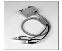
Terminal Connector: 4-Terminal Pair, BNC DUT Connection: 4-Terminal Cable Length (approx.): 1m (from connector to clip's tip) Weight (approx.): 260 g Additional Error: The additional error is negligible when compared to the instrument's accuracy. **Description:** This test fixture can measure lead components with low impedance. It has excellent repeatability and low contact resistance. It is equipped with two insulated Kelvin clips.
