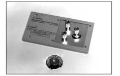
Terminal Connector: 7 mm DUT Connection: 2-Terminal Electrical Length: 3.4 mm Dimensions (approx.): 150(W) x 70(H) x 80(D) [mm] Weight (approx.): 175 g Additional Error: See figure below
