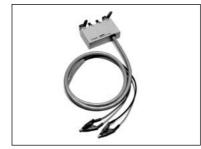
Terminal Connector: 4-Terminal Pair, BNC DUT Connection: 4-Terminal Cable Length (approx.): 0.94m (from connector to clip's tip) Weight (approx.): 300 g Additional Error: The additional error is negligible when compared to the instrument's accuracy. **Description:** This test fixture makes it possible to measure odd-shaped components that cannot be measured with conventional fixtures. It is equipped with two insulated Kelvin clips.
