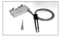
Terminal Connector: 4-Terminal Pair, BNC DUT Connection: 2-Terminal Cable Length (approx.): 1m (from BNC connectors to the top of tweezers) Weight (approx.): 290 g
