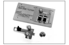
Terminal Connector: 7 mm DUT Connection: 2-Terminal Electrical Length: 3.4 mm Dimensions (approx.): 150(W) x 70(H) x 80(D) [mm] Weight (approx.): 180 g Additional Error: See figure below
