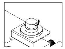
Remove the cap of the fixture
