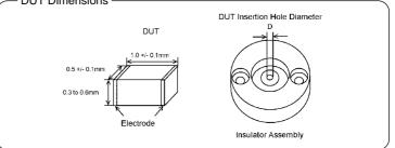
The 16196B is furnished with three different insulator assemblies, since any gaps between the DUT and the cylindrical insulator will result in improper positioning and subsequent measurement errors. Select an insulator assembly that reduces the gap the most. See the table below for dimensions of the insulator assemblies.
