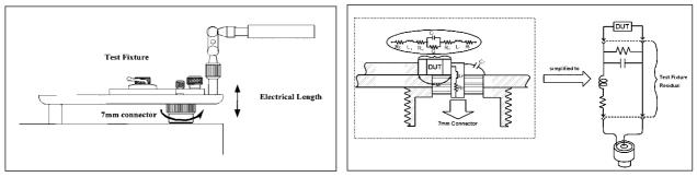
Electrical length of a test fixture
