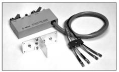
Terminal Connector: 4-Terminal Pair, BNC Cable Length (approx.): 1m (from connector to cable tip) Cable Tip: SMC (female) Weight (approx.): 250 g Additional Error: For detailed information, refer to the measurement instrument's specifications. **Description:** The test leads extend the measurement port with a 4-Terminal Pair configuration. It is provided with a BNC female connector board to allow the attachment of user-fabricated test fixtures.
