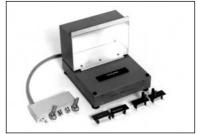
Terminal Connector: 4-Terminal Pair, BNC DUT Connection: 4-Terminal External Bias Input connector: High Voltage BNC(f) Dimensions (approx.): 180(W) x 120(H) x 200(D) [mm] Cable Length (approx.): 40 cm Weight (approx.): 1500 g
