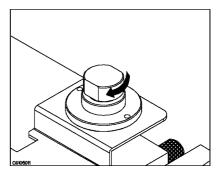
Replace the cap by screwing tightly
