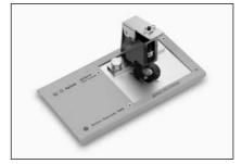
Terminal Connector: 7 mm **DUT Connection:** 2-Terminal Electrical Length: 14 mm Dimensions (approx.): 160(W) x 70(H) x 86(D) [mm] Weight (approx.): 300 g **Additional Error:**
