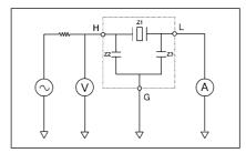
Guarding technique of an impedance measurement instrument
