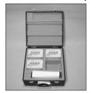
**Terminal Connector:** 4-Terminal Pair, BNC **Dimensions (approx.):** 142(W) x 88(H) x 112(D) [mm] (capacitors)
