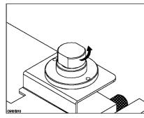
Remove the cap of the fixture
