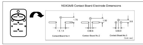
Electrode configuration for 16043A/B contact board
