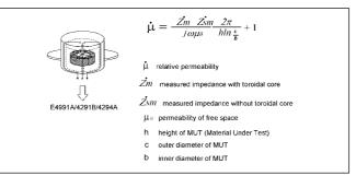
Permeability measurement method of 16454A
