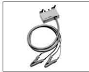
Terminal Connector: 4-Terminal Pair, BNC DUT Connection: 4-Terminal Cable Length (approx.): 0.94m (from connector to clip's tip) Weight (approx.): 300 g Additional Error: The additional error is negligible when compared to the instrument's accuracy.
