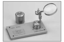
Terminal Connector: 7 mm **DUT Connection:** 2-Terminal Electrical Length: 27.3 mm **Dimensions (approx.):** 140(W) x 48(H) x 78(D) [mm] Weight (approx.): 250 g Additional Error:
