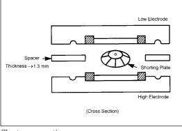
**Compensation and Measurement:** Open (Air-Capacitance) and short compensations are recommended in combination with the cable length compensation before measurement. First, set the instrument's cable length compensation function to 1 m. Then, short compensation is performed by using the furnished shorting plate. Open compensation is not performed, but its values are used in the dielectric constant equation as shown below:
