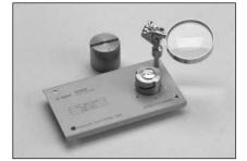
Terminal Connector: 7 mm **DUT Connection:** 2-Terminal Electrical Length: 26.9 mm Dimensions (approx.): 140(W) x 48(H) x 78(D) [mm] Weight (approx.): 250 g **Additional Error:**
