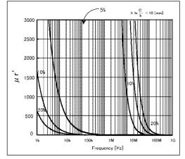
Typical Permeability (µr') Measurement Accuracy (@ h\* ln c/b = 10)
