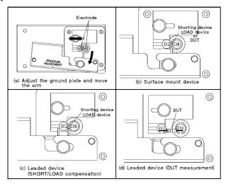
Placing the device
