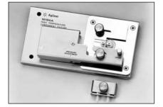
Terminal Connector: 7 mm DUT Connection: 2-Terminal Electrical Length: 50 mm Dimensions (approx.): 150(W) x 40(H) x 80(D) [mm] Weight (approx.): 350 g Additional Error: SMD:
