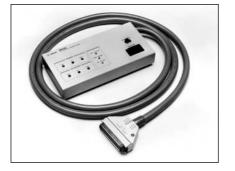
Terminal Connector: Handler Interface Cable Cable Length (approx.): 1.5 m Dimensions (approx.): 200(W) x 40(H) x 100(D) [mm] Weight (approx.): 800 g **Description:** The 16064B is designed to operate specifically with 4263A\*/B, 4338A\*/B, and 4339A\*/B. Comparator results which are sent from the measurement instrument, are displayed by LEDs on the 16064B. The parameters that are displayed are shown in the table below:
