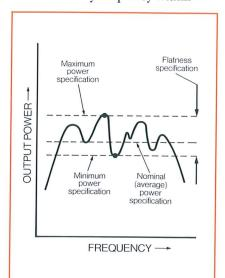
the bandwidth. The graph illustrates the differences that can exist in power claims for a given amplifier.
