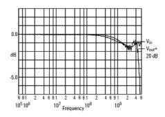
Figure 3.11. Notice how closely output matches input. Graph shows V<sub>in</sub> and V<sub>out</sub> when driven from a 25  $\Omega$  source.
