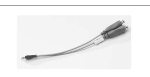
12 GHz Hi-BW solder-in differential probe head provides maximum bandwidth and minimizes capacitive loading to  $\leq$  210 fF. Variable spacing from 0.2 to 3.3 mm (8 to 130 mills).
