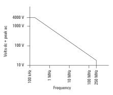
Figure 6.4. Derating curve showing bandwidth characteristics of the 10076A probe.
