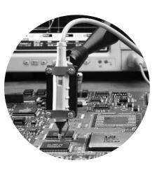
Figure 3.2. Agilent 1156A/57A/58A active probes for signals up to 4 GHz.
