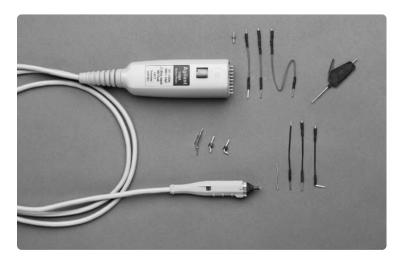
Figure 3.9. Agilent 1156A/57A/58A active probe for hi-speed signals.
