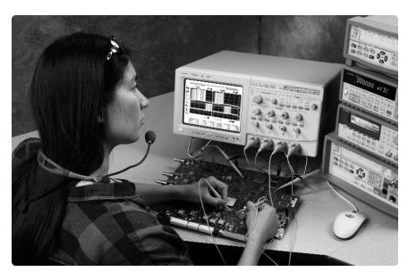
Figure 11.1. VoiceControl allows you to control the scope hands free.
