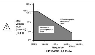
The above curve only applies to 10 MQ, 10:1 probes with the oscilloscope's input impedance set to 1 MQ.
