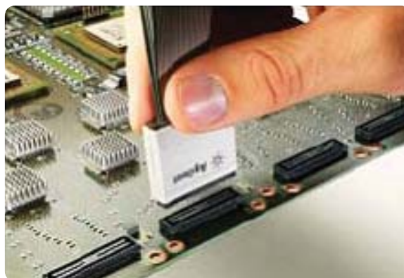
E5385A 34-channel Samtec connector probe
