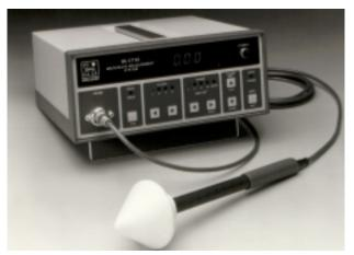
The RS232 interface allows easy adapting of the unit to computerized data acquisition in laboratory studies and semi-automatic production test systems. Digital Peak-Hold and Push Button Zeroing aid in improving testing productivity and reducing errors.
