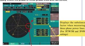
Display the fundamental voltage waveform for the 1st order (U1, U2, and U3) as a phase angle of 360° as a standard. Ideal for checking three-phase power lines
