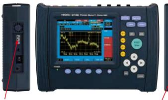
External event input/output terminals Event output : Outputs a signal when events occur-either as an
