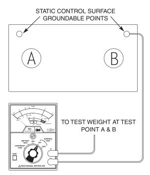
Figure 5-4: Material Evaluation Surface to Groundable Point Test
