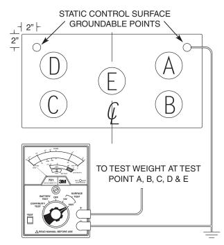
Figure 5-1: Periodic Performance Tests of Installed Surfaces
