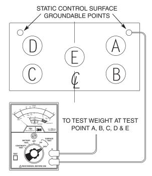
Figure 5-2: Qualification Tests of Installed Surfaces
