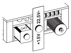
Figure 6-1: Battery Replacement
