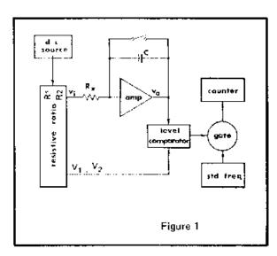
The basic block diagram of the system is shown in Figure 1 where  $R_{\mathbf{x}}$  denotes the high resistance under test. Operation is based upon an analog integration technique employing a high quality, solid state electrometer and a feedback capacitor C.
