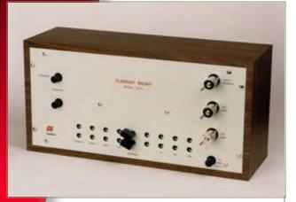
**G** uildline Model 9211A is a four-terminal bench top or rack mount instrument designed for convenient measurement of current in nine ranges from 10 microamperes to 300 amperes. Voltage output at full rated current on all ranges is 0.1 volt. Accuracy is calibrated at 23 °C, and referred to the unit of resistance as maintained by the National Research Council of Canada or the National Institute of Standards and Technology. A report of calibration giving the measured values is furnished.
