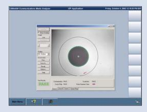
human eye, the VIP application eliminates the possibility of injury as with traditional connector microscopes.
