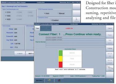
Designed for fiber installation and commissioning, Construction mode eliminates the time consuming, repetitive tasks of parameter selection, analyzing and file saving. A wizard guides the
