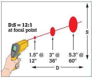
Use the Fluke 63 within six feet of the intended target. At greater distances, the measured area will be larger (approximately the distance divided by 12). The Fluke 63 offset single-point laser indicates the approximate center of the measurement area.
