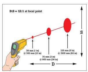
When measuring smaller objects, use the Fluke 561 within 6 ft. (1.75 m) of the intended target. The measured area increases with distance (the distance divided by 12, approximately).
