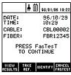
Organize test results using alphanumeric identifiers that directly reflect your cable and fiber identification system.
