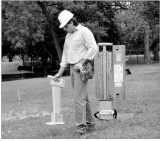
The Dynatel 2273 Advanced Cable/Fault Locator can be used with the Dynatel 2205/2206 EMS Marker Locating Accessory.
