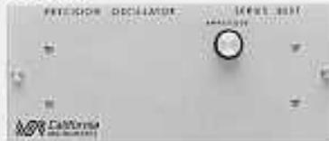
The model 855T is designed for those applications where access to the frequency adjustment is to be limited. Frequency changes are by means of an internal DIP switch which can be set from 45Hz to 9999Hz. Amplitude adjustments are by a front panel control (optional "locked" amplitude control is available).
