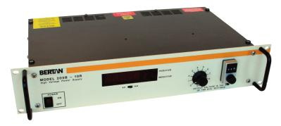
Spellman's Bertan brand of 205B Series high voltage power supplies provide regulated high voltage outputs from 1 to 50kV. The low noise, linear topology employed results in extremely low output ripple specifications. These 15 to 30 watt units are inherently reversible by design, providing either positive or negative output polarity. The 205B is fully arc and short circuit protected. Excellent regulation specifications are featured along with outstanding stability performance.
