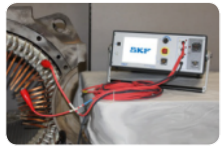
A Baker DX-15A testing individual stator coils.
