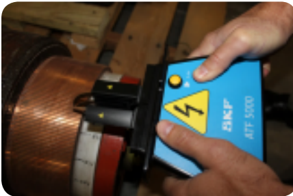
The ATF 5000 DC armature test accessory comes bundled with the Baker DX-15A.
