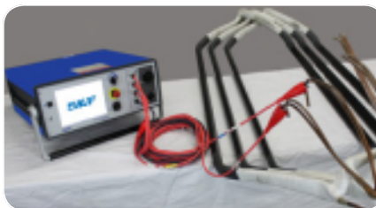
The Baker DX-15A as a coil test analyzer.
