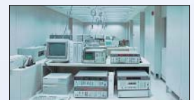
Temperature- and humidity-controlled calibration room
