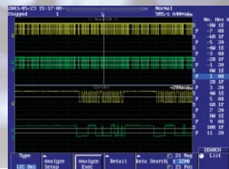
Analysis results of 6.4 seconds of I 2 C data.
