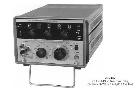
The 2553 is an ultra-stable, high-resolution DC voltage and current source which delivers output voltages from 1  $\mu$ V to 12 V, and output currents from 0.1  $\mu$ A to 120 mA at an accuracy of ±0.02%.
