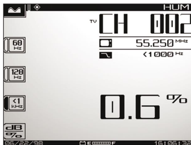
In-service "HUM" (PAL and NTSC compatible)
