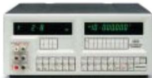
DC & AC Voltage, DC & AC Current and Ohms. Calibration of DMMs to 8-1/2 digits.
