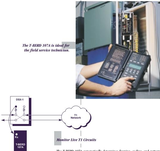
The T-BERD 107A automatically determines framing, coding, and pattern. Errors are detected and displayed at a glance on the front panel. Monitor signal quality or view data bits on any DSO channel. Decode the SLC datalink or ESF signal and monitor signaling bits to troubleshoot problems in the field.
