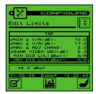
▲ The MS1400 has a limit set for analog channels and a limit set for digital channels.
