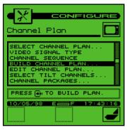
working. It's only necessary to build a channel plan once. A "cloning" function makes it possible to easily transfer channel plans from one field instrument to the other. StealthWare™ software enables you to upload and download channel plans from your PC to the meter (MS1300, MS1400).
