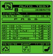
Auto Test results are time, date, and temperature stamped and can be stored, viewed, printed or uploaded to StealthWare software (MS1300, MS1400).
