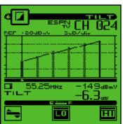
The tilt display provides a display of six channels that updates in less than a second (MS1200, MS1300, MS1400).
