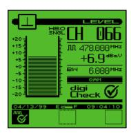
▲ The digiCheck™ method of measuring the total integrated RF-power under the haystack is very reliable and accurate. All level readings are fully compensated for by the correct occupied bandwidth.
