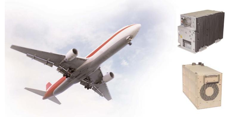
TDI's Airborne DC/AC Sinewave Inverters are fully compliant to RTCA/DO-160D Environmental and EMI criteria for Instrumentation and Emergency Power applications. These products provide a clean (< 2% THD), regulated 400Hz electrical bus from APU or Battery (DC) power sources. Our internal "air tunnel" cooling technology shields sensitive electrical components from exposure to adverse environmental conditions.
