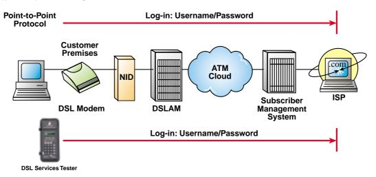
The DSL Services Tester ensures a successful point-to-point protocol connection from the customer to the ISP.
