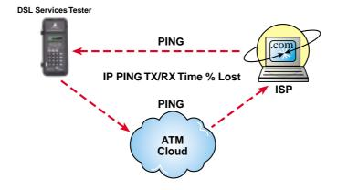
The DSL Services Tester verifies IP layer routing.
