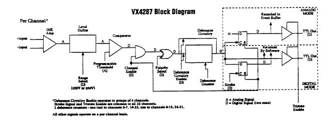
Figure 1: VX4287 Block Diagram
