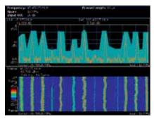
Here, a Frequency Mask Trigger was set to monitor the frequency domain any changes in the spectrum and it triggered on transient interference. The spectrogram shows the time relationship between the wanted good signal and the interference transient signals and the spectrum display shows what was happening at the precise moment the interfering signal was present in the band. FMT is an essential tool for separating known signals from unwanted interference.
