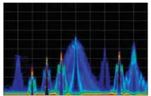
Revolutionary DPX display discovers transients, instability and glitches that other analyzers miss. Here, an RFID interrogator and tags are seen transmitting at different power levels and frequencies.
