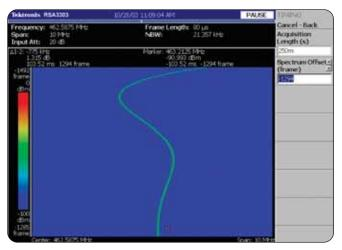
RSA Series Spectrogram uniquely shows time-varying signal behavior in frequency change/stability, spectrum occupancy, pulsed signal timing, power change and more! The sample on this page shows the frequency settling characteristic of a transmitting device.
