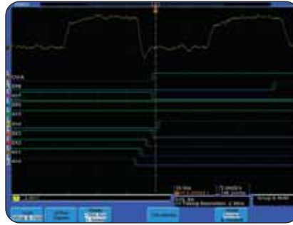
► Multi-channel setup and hold triggering highlighting multiple violations (MSO4000).
