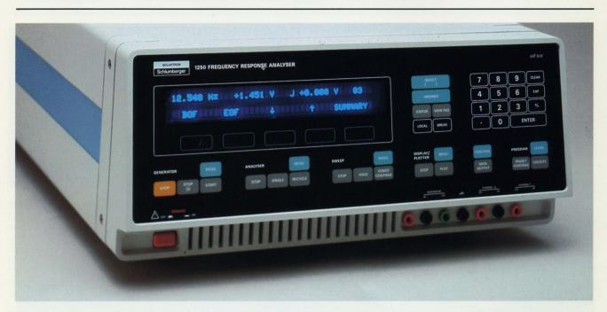
The 1250 series Frequency Response Analyzers use the single sine correlation analysis technique to provide fast and precise measurement of the amplitude and phase characteristics of the device under test. The device can be stimulated with a sine, square or triangular waveform from the built-in generator. For self-excited devices, the 1250 can be synchronized to an external reference to determine the harmonically related response characteristics.
