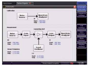
The following parameters can be measured at a specified frequency or in a selectable frequency range: Noise figure in dB
