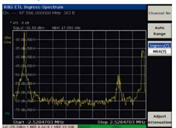
Frequency spectrum of a J.83/B-signal with interferer.
