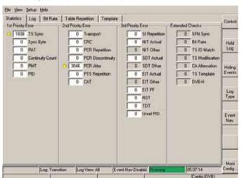
In digital television (DTV), pictures, sound and additional information are transmitted as a digital MPEG-2 transport stream. The MPEG-2 transport stream's complex structure must conform to defined rules so that it can be properly processed by the receiver. A range of MPEG options can be added to the R&S°ETL to analyze the structure of MPEG-2 transport streams in addition to the RF quality of DTV signals.
