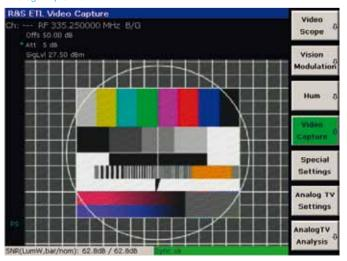
The R&S°ETL standard version comes with a range of elementary measurements for analyzing analog TV signals. The video analyzer functionality needed at the transmitter site or at the cable headend can be added to the R&S°ETL.
