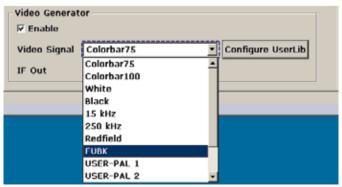
Often, high-quality reference signals are needed to reproducibly check and accurately measure the transmission characteristics or simply test the functionality of transmitters and modulators. The need for a separate signal generator has now been eliminated. Remaining true to the all-in-one motto, the R&S°ETL again offers the ideal solution, with integrated analog and digital signal generators.
