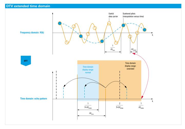
A special feature of the R&S<sup>®</sup>ETL is the positioning of the FFT window. To help ensure stable synchronization to the transmitter signal, especially for field measurements, the R&S®ETL tries to place all impulses above an echo detection threshold so that they are equidistant within the guard interval. For some applications, the echo detection threshold is dependent on the system optimization method selected by the user.
