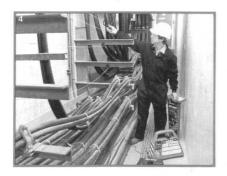
**Extension rod** (5) 70cm/28in long enables the signal clamp, the clamp antenna or the small stethoscope to be applied to an overhead line or to a cable in a deep vault. Up to three extension rods can be joined together.
