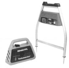
Fault Finder is a classic A frame to pinpoint damage or breaks in a buried cable sheath. The Fault Finder is a complete self contained unit for cable tracing and for locating sheath faults up to 1.5 MOhms. The transmitter needs an additional mode for use with the Fault Finder; specify the RD400FFL transmitter which is suitable for use with both the RD400 locator and Fault Finder. See data sheet 220.
