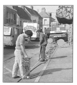
The locator comprises a handheld receiver and a signal transmitter. The transmitter applies its signal to a buried metal pipe or cable which is then located and traced with the RD400 receiver. The receiver also has two more detection modes used without the transmitter, for locating signals occurring 'naturally' on buried conductors.
