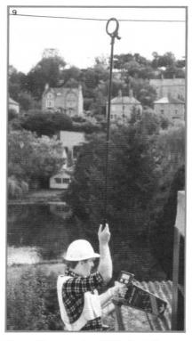
**Live cable connector** (8) Similar to the plug connector but specially insulated clips are suitable for connecting directly to conductors of low voltage live cables, For use only by qualified personnel. See data sheet 110.
