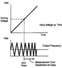
Voltage-controlled oscillators can be dynamically tested by measuring frequency at given voltage points. The sample time can be made as small as two periods of the incoming signal. Resolution then can be increased by averaging a number of measurements.
