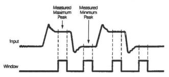
An additional arming capability, Synchronous Window Auto-Trigger, allows auto-trigger to operate only within a specified "window". This window can be set, for example, between possible ringing on both the rising and falling edges of the signal. Measurements are then performed during this window, resulting in far more accurate measurements than would otherwise be obtained.
