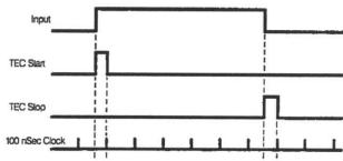
TEC improves resolution by initiating a pulse at precisely the same time as the START edge, and a second pulse precisely at the STOP edge. The pulse width of these error signals is set by the next clock pulse. Even pulses with durations smaller than the internal clock can be evaluated using this method. The action is similar to that shown in the chart above.
