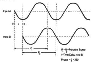
The 1995 and 1996 automatically measure the phase differential between two signals. Phase measurement involves three automatic measurements: Ratio, to assure that A and B are at the same frequency; the Time Interval between the two signals: and Period.
