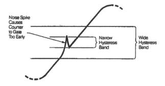
To overcome hysteresis limitations, Racal-Dana offers two bands: a narrow one to reduce trigger level timing errors on noise-free signals, and a wide one which may be used on extremely noisy signals. The standard hysteresis band is 25 mV; the high-level band is 100 mV.
