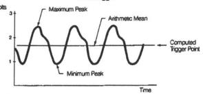
In the auto-trigger mode, the counter measures the input signal's maximum and minimum peak voltages. The microprocessor sets the trigger levels at the computed mean. With continuous auto-trigger, the mean is recomputed upon any change in signal amplitude or offset. The attenuator is selected automatically to permit measurement of any input waveform within the instrument's full ±250 V operating range.
