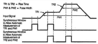
Automatic rise time and pulse width measurements on complex pulses can now be made. In conjunction with Synchronous Window Auto Trigger, the above waveform can be fully evaluated. This type of signal is often found in Electronic Warfare systems—in video log amplifiers, for example.
