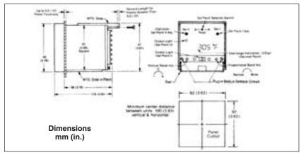
Option "T" (Triac): Solid state plug-in triac rated 1 amp holding and 10 amps in-rush
