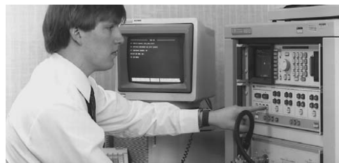
Figure 3. Engineer evaluating design at the HP8510B ANA
