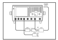
The diagram shows the set up required to characterize a voltage controlled oscillator (VCO). This is achieved by determining the maximum and minimum frequencies of operation, the frequency linearity and measuring the output power against tuning voltage of the device. The unique capability of the 6200B series MTS to measure frequency against tuning voltage of a VCO speeds up production test and reduces bench clutter.
