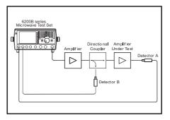
Test Set up for Ratioed Measurements
