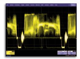
understand approximate behavior. WaveStream makes it easy to understand jitter on edges or in eye diagrams. WaveStream also excels in allowing you to relate composite (WaveStream) to single-event (real-time sampled) behaviors. Just capture in WaveStream mode, toggle to view or zoom a single trace, then toggle back to WaveStream mode.
