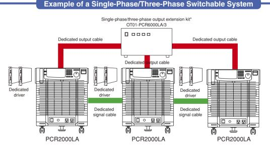
\* The output extension kit (option) includes all the components necessary to implement this system configuration, including dedicated drivers, output cables, and signal cables.
