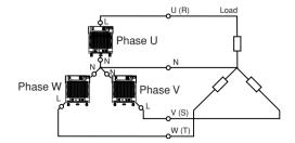
• Parallel extended operation system using three phases \* Three-phase operation is possible with each phase operating in parallel.
