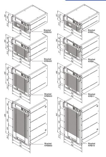
For metric-type racks (JIS) KRB250 (for PCR500LA) KRB400 (for PCR1000LA) KRB500 (for PCR2000LA) KRB850 (for PCR4000LA)
