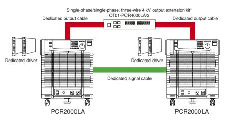
\* The output extension kit (option) includes all the components necessary to implement this system configuration, including dedicated drivers, output cables, and signal cables.
