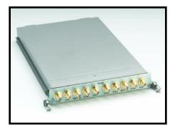
The Model 7712 plug-in module offers a  $50\Omega$ , dual  $1\times4$  multiplexer configuration with rear panel SMA  $1\times4$  connectors. Multiple multiplexers can be cascaded to build scalable matrix and multiplexer systems for a large number of
